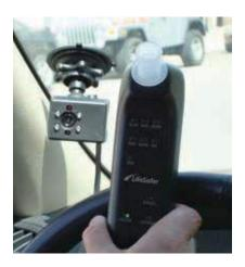
The LifeSafer FC100 with Camera System Handset is controlled by the Camera. The Camera must detect your image and "see" the target on the back of the Handset before it will allow you to take a test. Hold the Handset 4-8 inches from the front of the Camera module in order to get the Camera to release the Handset for the test.
