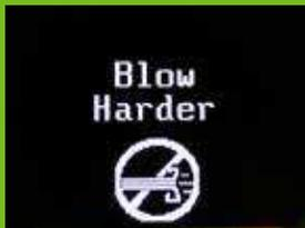
This abort explanation means that the breath sample delivered was insufficient.
