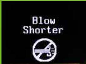
This is one of the Abort explanation screens and means that you have blown longer than the required time.
