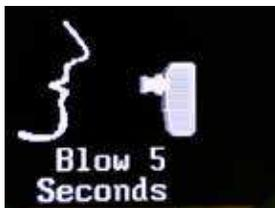
To successfully complete a test you will need to blow into the mouth piece long enough and with sufficient pressure while generating a hum tone created by saying the word "DO" as you blow. Once you start to blow and hum the device will emit a continuous tone which will stop once you have completed the test.
